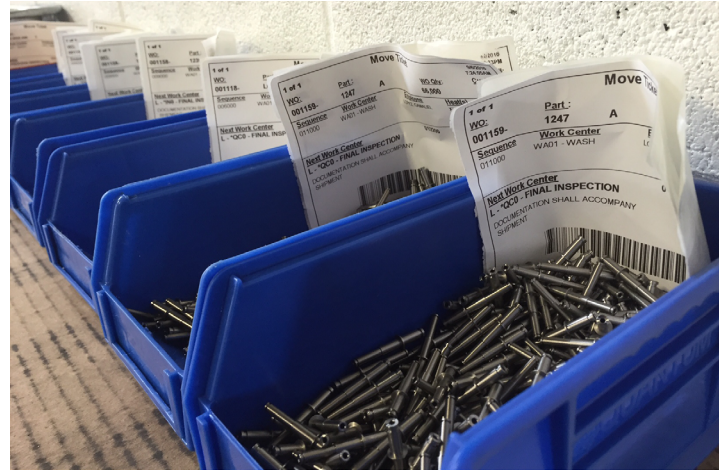
Move tickets identify where the parts have come from and where they are going for the next operation.
